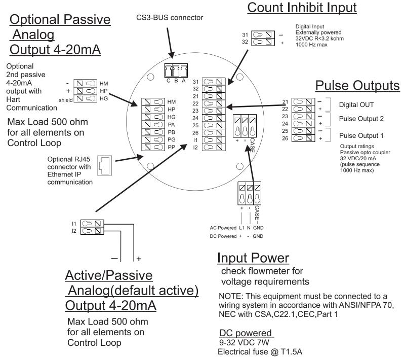
AC powered 100-240 VAC 50/60HZ Electrical fuse @ T500mA
